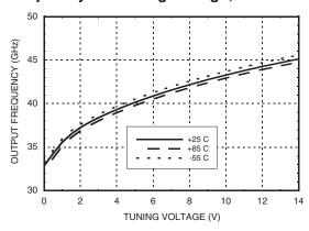
Frequency vs. Tuning Voltage, T = +25°C
